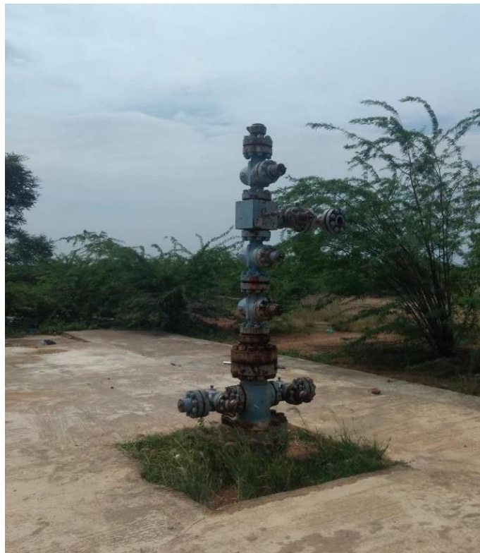
Figure 1: Christmas tree of the exploratory well in Karukkakurichi, a village near Neduvasal.
