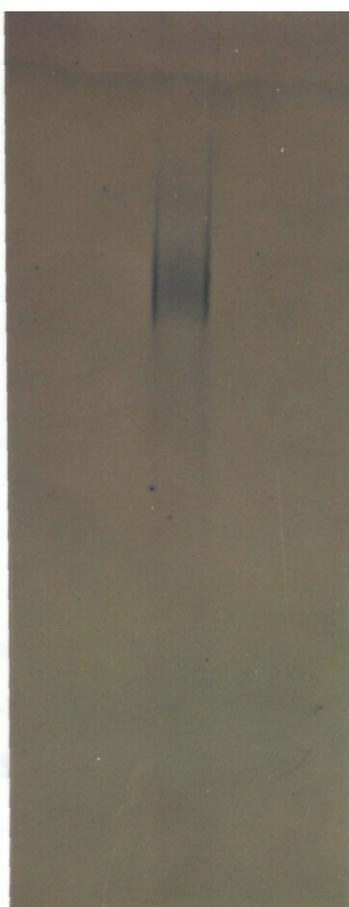
Fig. 5: Iron specific staining of ferritin was carried out by soaking the 5% Native PAGE in 2% potassium ferricyanide in 50% ethanol and 7% acetic acid for 4 hrs. Note the Prussian blue colour of ferritin.
