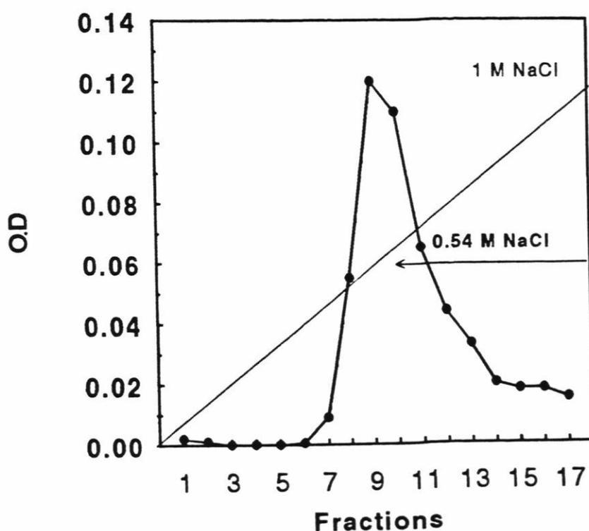
Fig. 4: Anion exchange chromatography of *V.mungo* ferritin on DE-52 column. 30% ammonium sulphate fractionated proteins were loaded on 50 mM Tris-HCl pH 7.5 equilibrated column and after washing with the equilibration buffer, the protein was eluted with linear salt gradient from 0-1 M NaCl. Absorbance of the fractions was recorded at 280 nm. Ferritin eluted at 0.54 M NaCl concentration. Fraction size 4 ml/mm.
