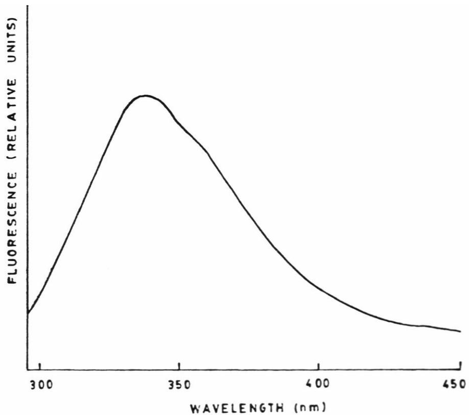
Fig. 11: Fluorescence emission spectrum of ferritin at room temperature showing peak at 340 nm. Excitation wavelength used was 286 nm, 5 nm band pass, 5 nm emission pass and instrument response of 2.
