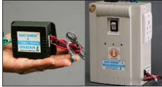
Fig. 3.26: Nano Ganesh: Distant Agriculture water pump can be controlled and monitored by a mobile phone. [460] [461] [463] [464]
