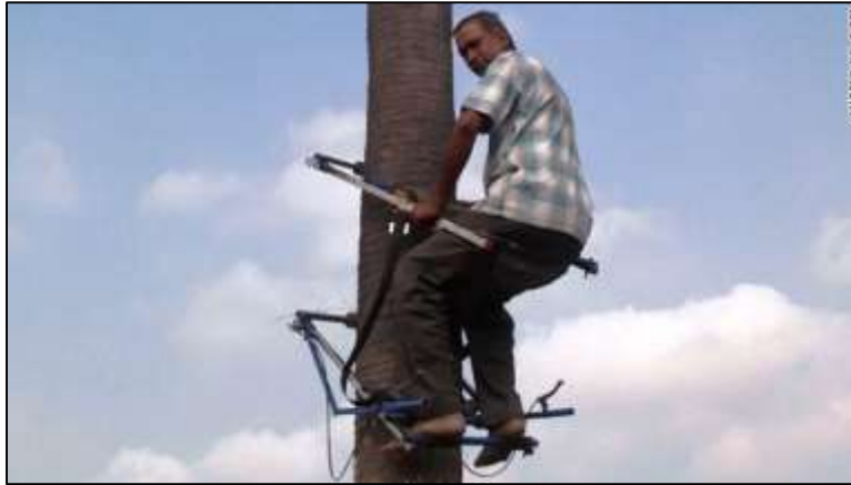
Fig. 15.32: Mechanical Tree Climber by D. Renganathan [82]
