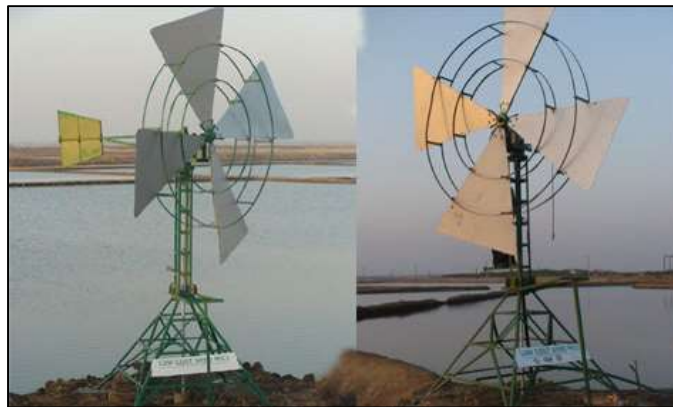
Fig. 15.55: Low-Height Wind Mill for Lifting Ground Water by Mehtar Hussain and Mustaq Ahemad [97]
