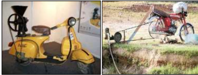
Fig. 15.66: Scooter Flour Mill by Mr. Sheikh Jahangir, Jalgaon India and Water pumps powered by motorcycles [90] [94]
