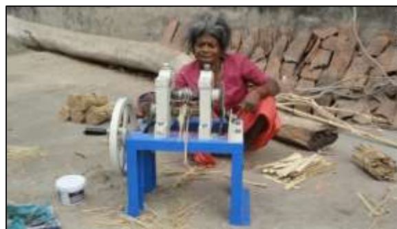
Fig. 15.39: Bamboo Splint-Making Machine by Paresh Panchal [82]
