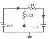
73. The forward voltage drop, Zener Voltage (Vz) and the maximum reverse current (I<sub>Zmax</sub>) of the Zener diodes in the circuit shown in the figure are 0.7 V, 9.3 V and 32 mA, respectively. The maximum value of the load resistance (R<sub>L</sub>) that can be used without exceeding I<sub>Zmax</sub> in any of the Zener diodes is
