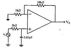
34. The output voltage of the circuit given below is approximately
