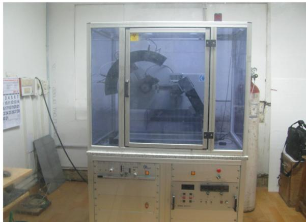
Fig. 2.1 INEL X-ray diffractometer.
