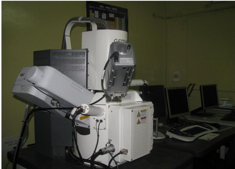
Fig.2.6 Field emission scanning electron microscope (model: Carl ZEISS, FEG, Ultra 55).
