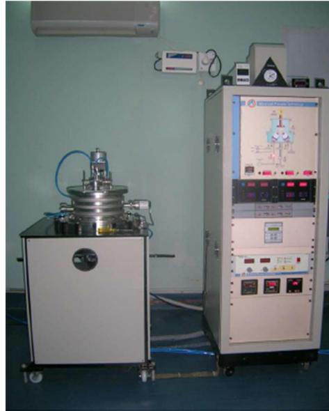
Fig.3.15. Sputtering system used in the present study to deposit Nickel films
