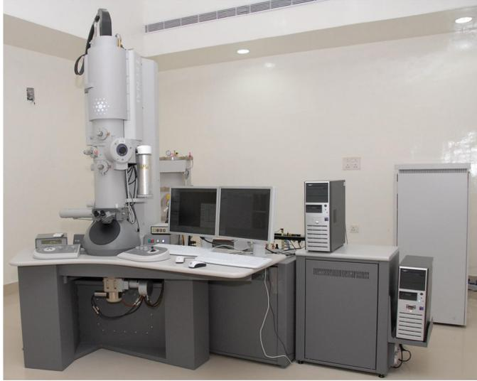
Fig. 2.7 Photograph of FEI Tecnai G<sup>2</sup> S-Twin, FEI Transmission electron microscope.
